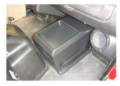
Place the enclosure on the passenger side footwell and lift the box onto the center hump, lift the driver side higher and slide in using a sidways motion
