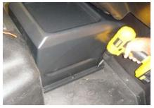
Once the enclosure is in place, screw the 6 mounting screws into the floor using a phillips screw bit in a cordless drill
