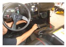
Continue sliding the box over the hump till it sits in place and makes good contact with the floorboard
